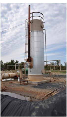
Many industrial and mining processes require chemical basins or lagoons — either for storage, secondary containment or processes such as solvent extraction. Plastatech OR (Oil Resistant) geomembrane is engineered to resist most chemicals — including oils, acid and alkalies as well as a wide range of chlorinated, aromatic and aliphatic hydrocarbons.
